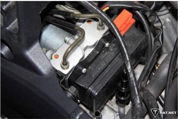
Above: on a Sprint the Nissin ABS ECU and Modulator Unit is located behind the engine next to the rear shock. Access is not required for brake bleeding.
